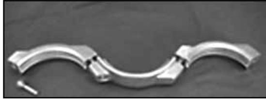
4. Tighten each bolt in sequence a few turns at a time maintaining an even gap between segments. Avoid pinching of the hose between the segments. A light solution of soapy water can be used as a lubricant between the hose and segments.
