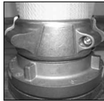
3. Lightly grease the bolt threads.
